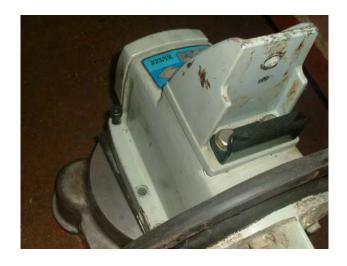
Bolt Volvo sail drive to mini flywheel housing using M10 cap heads and M10 nylock nuts provided.
