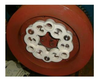
Fit rear part of drive plate and element to flywheel inertia ring. Inertia ring 201-00847 Drive plate 206-04108 For BD902 (BETA 25) use inertia ring 201-06595
