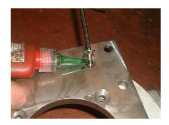
Bolt Volvo adapter (201-01737) to mini flywheel housing (201-01738) using M8 counter sunk screws provided with thread lock. (This may have already been finished for you).
