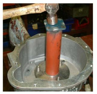
Align spline and knock front part of drive plate onto shaft of sail drive. Fit until the plate is **76mm** from point A to point B.
