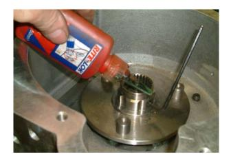
Once plate is in position, lock grub screw onto shaft using small amount of thread lock.
