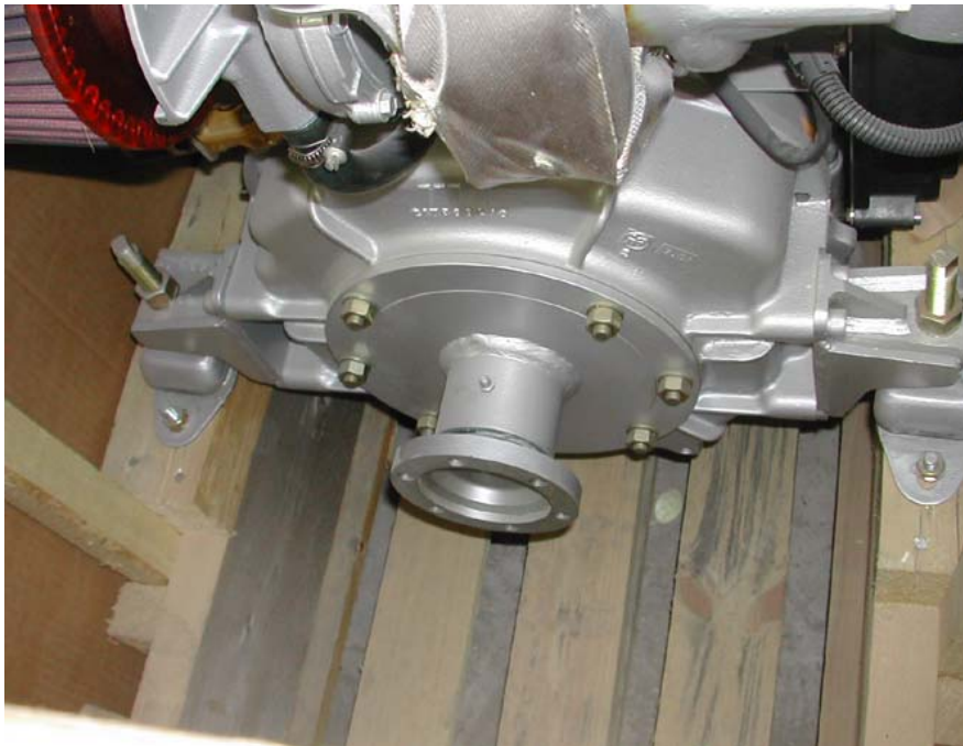
Bobtail adaptor for installations without gearbox.
